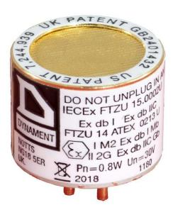
Dynament infrared sensors operate by using the NDIR principle to monitor the presence of the target gas. The sensor contains a long life tungsten filament infrared light source, an optical cavity into which gas diffuses, dual temperature compensated а pyroelectric infrared detector, integral an semiconductor temperature sensor and electronics to process the signals from the pyroelectric detector.
